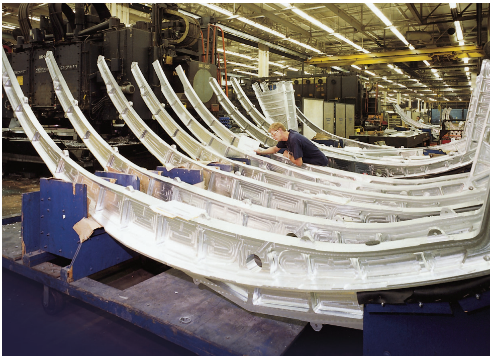
An employee of the St. Louis GKN Aerospace manufacturing facility inspects machined aluminum-alloy aircraft ribs.
