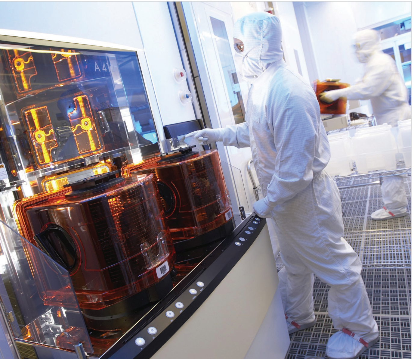
Electronic Materials strengthen silicon wafers at an annealing furnace at the company's plant in St. Peters, Mo., near St. Louis.
